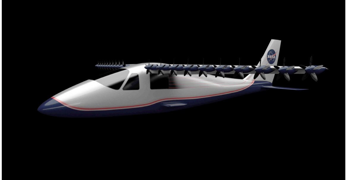
ESAero's Scalable Convergent Electric Propulsion Technology Operations Research (SCEPTOR) technology is being used by NASA to explore the system level impacts of distributed electric propulsion // Photo courtesy of NASA //
