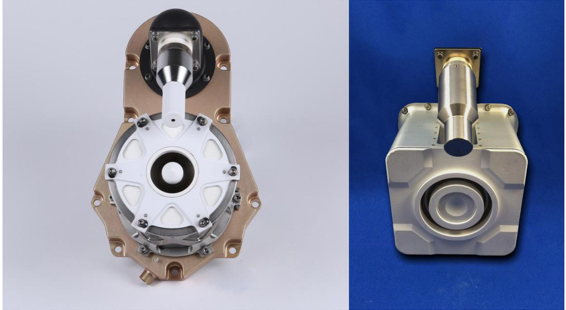
LEFT The Busek BHT-200 was the first U.S. developed Hall Effect Thruster to fly in space (TacSat-2, 2006)
