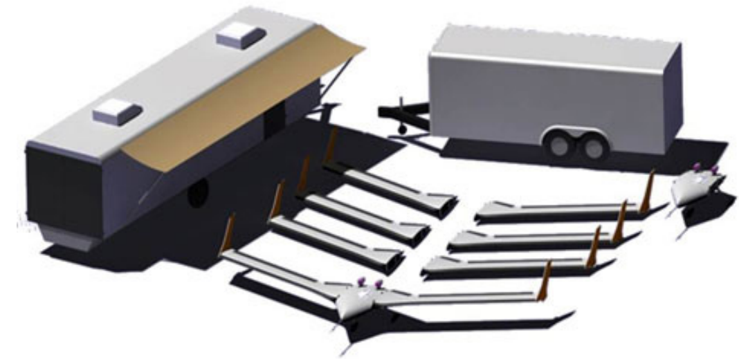
Artist's rendering of X-56A MUTT package, consisting of the aircraft with three additional wing sets and a second fuselage/mid-body (center), flanked by the ground control station on the left and the air vehicle storage/transport trailer on the right. (AFRL/Lockheed image)
