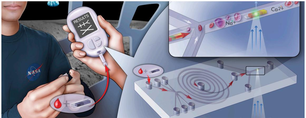
DMI's test strips, the size of 165 by 33 micrometers, are produced to handle a microliter (tiny drop) of blood. To get an idea of the scale of the strip, the width of a single human hair ranges from approximately 10 to 200 micrometers. The nanostrips each have the mass and volume at the nano range, occupying no more than the volume of a few blood cells.
