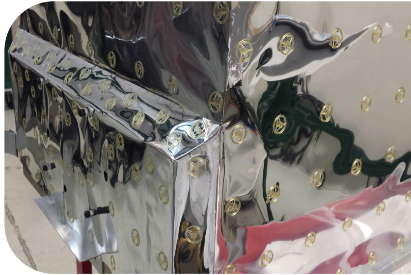
Quest's IMLI uses discrete micro molded polymer spacers to separate layers of insulation
