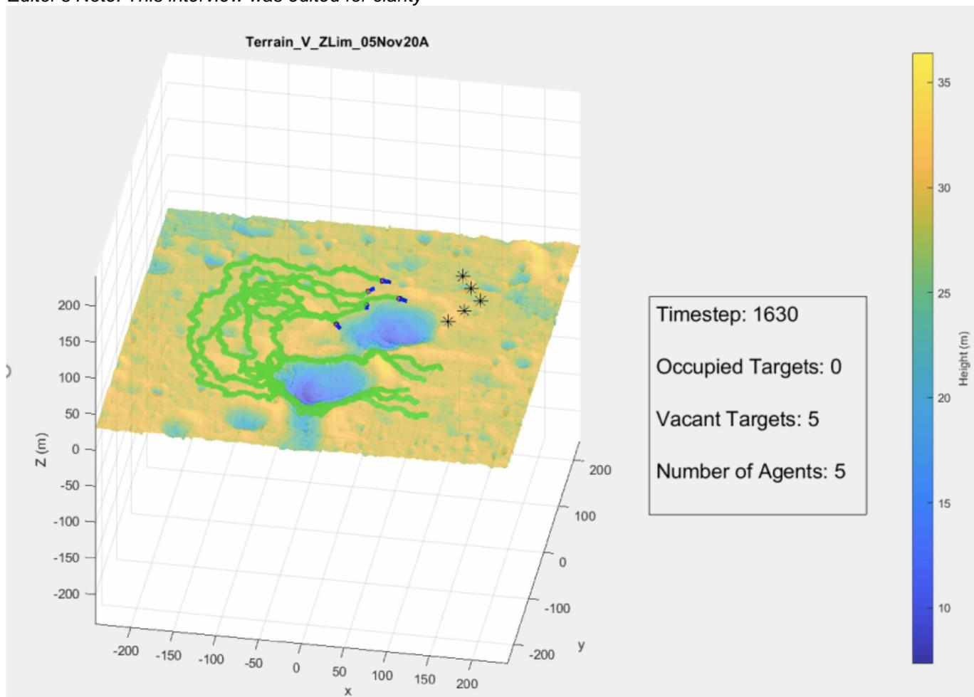
Example output of the SWARM Toolset developed under the NASA SBIR/STTR program. Photo credit: ASTER Labs, Inc.
